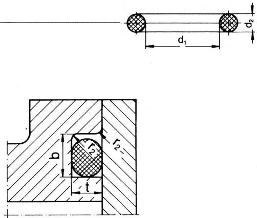
The measurement »b«, which is the width of the O-Ring groove, has to be larger than the deformed O-Ring. Depending upon application the groove may be open on one side. However, the pressure applied to the medium to be sealed must have full access to the O-Ring. The surfaces of the groove and the opposed surfaces should have more or less rounded processing traces to permit peak-to-valley-heights of 44 — 25  $\mu\text{m}$ .
