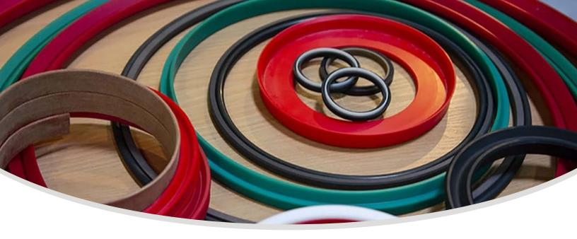
O-rings are among the most commonly used seals across various applications due to their low cost and reliability. An O-ring is a round gasket with simple mounting requirements, designed to sit in a groove and be compressed between two or more parts. The compression during assembly creates a seal that prevents liquids or gasses from entering or escaping.
